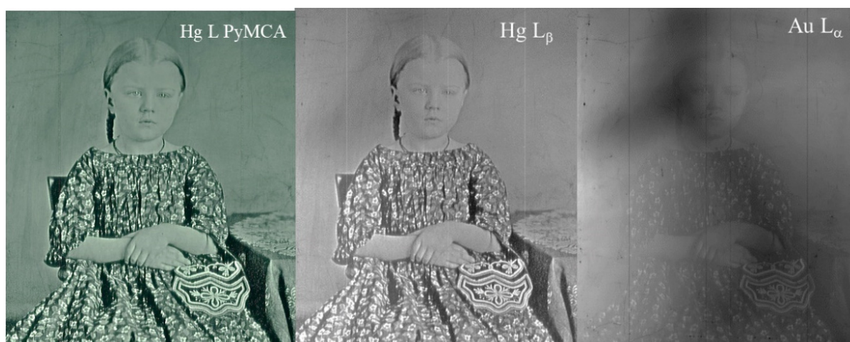
Figure 6. XRF image from left to right using the Hg L PyMCA fit, and Hg L_{\beta} and Au L_{\alpha} without fitting.
