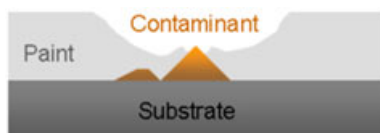
Figure 2. Illustration of paint crater formation caused by a contaminant with low surface energy, from which the applied paint is displaced.
